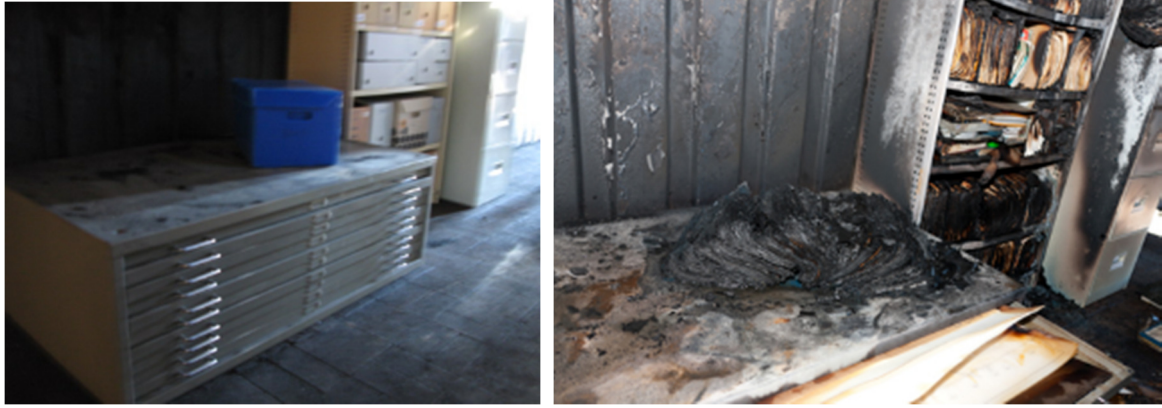
65 & 66. EXPOSED FLUTED POLYPROPYLENE BOX (STAMINEX) - BEFORE AND AFTER
