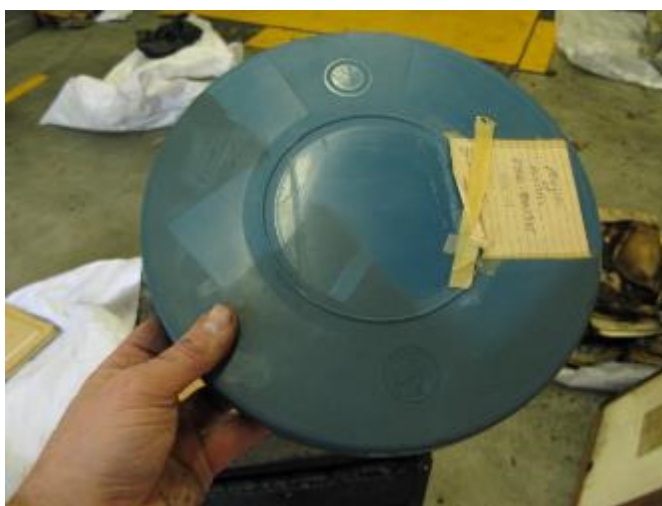
54. POLYPROPYLENE FILM CAN — BROWN DEPOSIT, POSSIBLY FIRE RETARDANT
