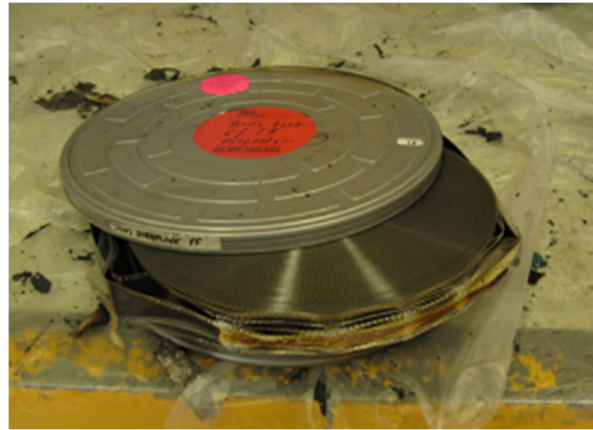
43 & 44. POLYESTER FILM IN STEEL CAN - BEFORE AND AFTER
