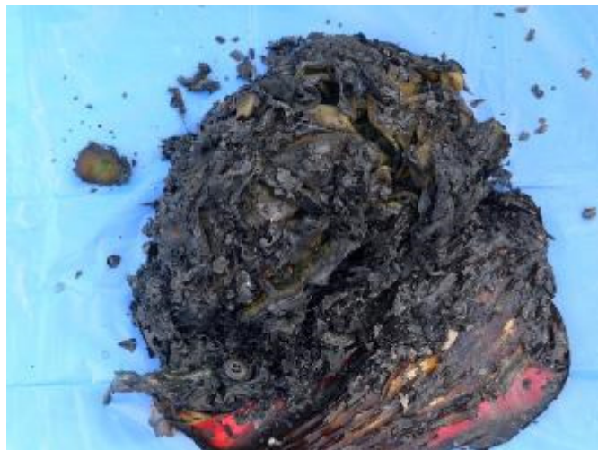
The Disruptive Pattern Camouflage Uniform jacket with cotton dust cover caught fire and fell on to the red file below. The cover was largely consumed and significant damage was done to the uniform itself.
