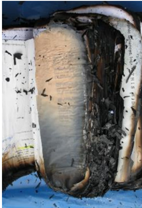
Thermo-fax paper on a file. The paper darkened where it reached a sufficient temperature.
